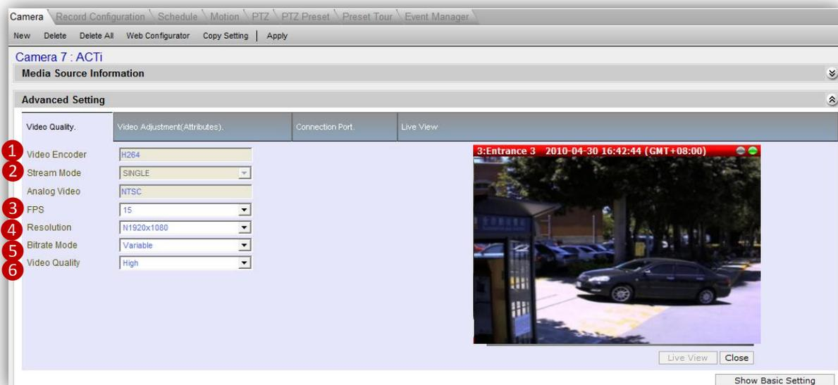
**Fig. 22 Camera Setup –Advanced Setting - Video Quality**
