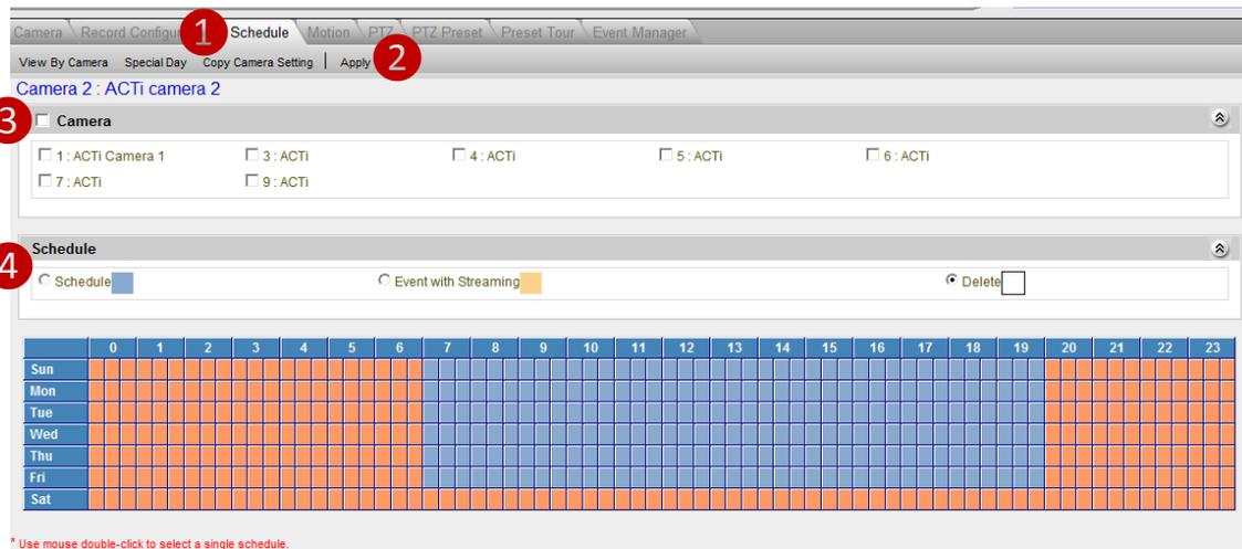
**Fig. 29 Camera Setup – Schedule – Copy Setting(Weekly)**
