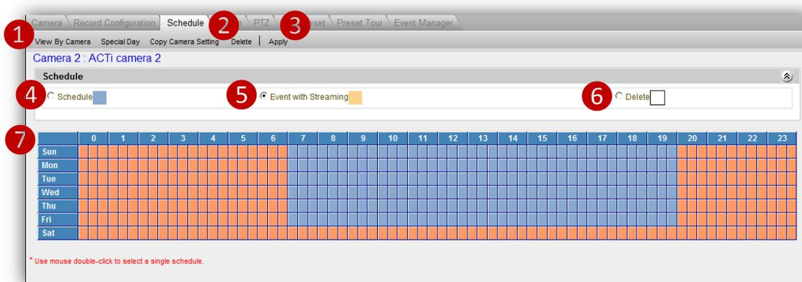
**Fig. 28 Camera Setup - Schedule – Weekly View**
